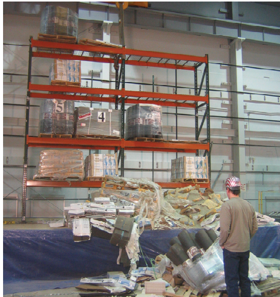
Figure 1 - Damage State DS1 for Storage Racks: Significant Merchandise Shedding (from Filiatrault et al. 2008).
