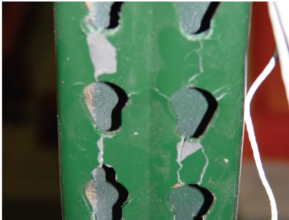
Figure 2 - Damage State DS2 for Storage Racks: Significant Structural Damage to Rack Structure, a) Buckling of Upright, b) Base Weld Fracture, c) Cracking and Tearing Across Down-Aisle Connector Perforations in Uprights and d) Damage to Beam Connectors (from Filiatrault et al. 2008).
